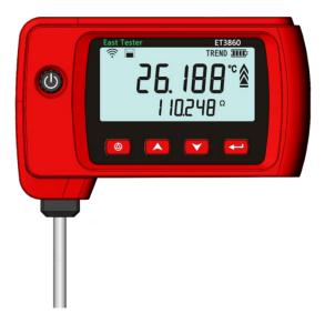
ET3860 Series Precision Digital Thermometer is a pprecise thermometer, which could replace mercury glass tube liquid (LIG) thermometers. The temperature measurement range is  $-80\sim450~^{\circ}\mathrm{C}$ . It also can be used as standard reference thermometer for other types of digital or anolog thermometers.
