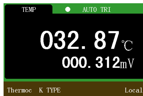
Figure 5-23 Thermocouple temperature measurement
