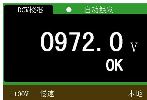
Figure 8- 2 DC voltage calibration is completed
