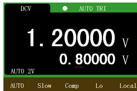
Figure 5-14 Lower limit setting interface
