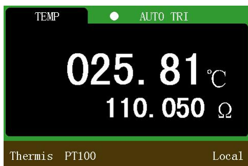
Figure 5- 18 Thermal resistance temperature measurement
