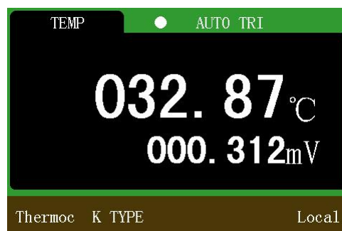
Figure 5- 19 Thermocouple temperature measurement
