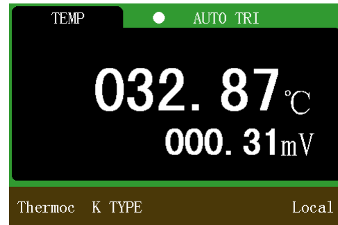
Figure 5-23 Thermocouple temperature measurement
