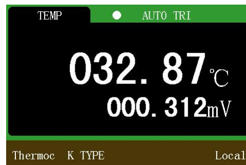
Figure 5-20 Thermocouple temperature measurement
