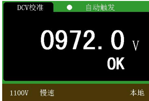
Figure 8-2 DC voltage calibration is completed
