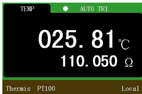
Figure 5-19 Thermal resistance temperature measurement
